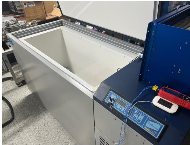
Rapid cooling chamber
