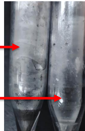
#Early Dirty ampoule Bad cracks
