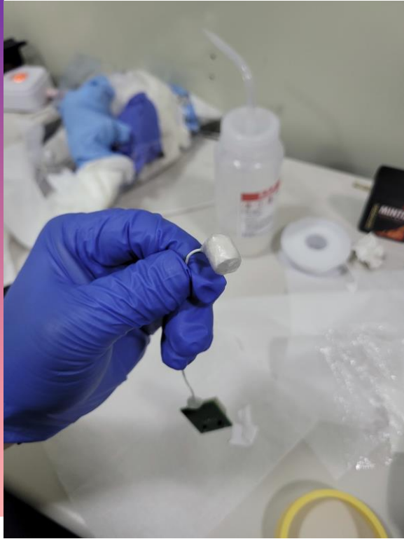
\text{CeBr}_3: ^{139}\text{Ce} Crystal with SiPM connection
