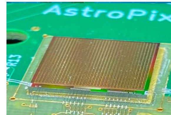
AstroPix tracking layers to capture 3D image of shower development NASAAMIGO-X mission
