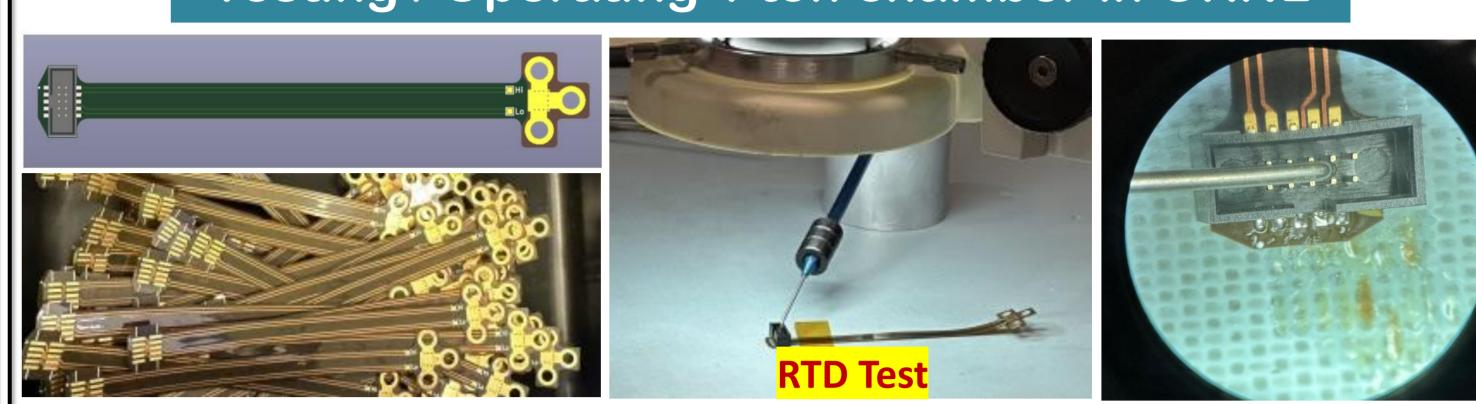
• We conducted calibration of RTD in ORNL to measure temperature in each area by putting it inside the Chamber.
