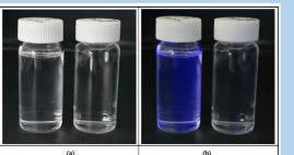
Light emission from (a) CbLS (left) and water (right) under visible light and (b) ultraviolet test conditions
