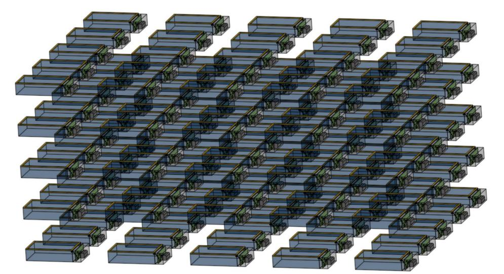
By stacking these detectors to form an X-Y-Z array (left) and using the coincidence between these detectors as a trigger, we obtain the 3D event rate and track info of cosmic muons.
