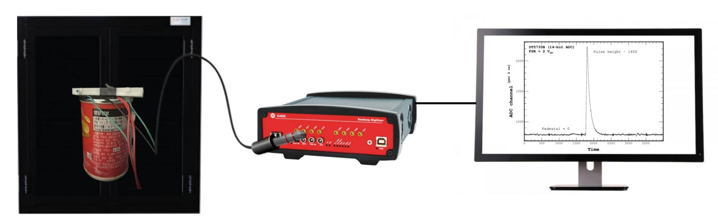
A typical example of a signal pulse (above), which is liberated from the detector then digitised by the CAEN DT5730 digitiser.
