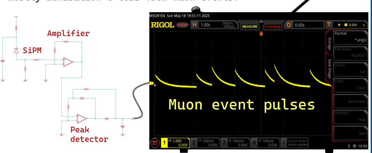
We have amplified and stretched the voltage pulse of muon events for further processing along the DAQ chain (Bottom right).
