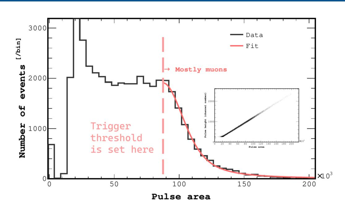
We verify the threshold on the electronics by identifying the most probable value of muon energy loss from the pulse area spectrum and is set low enough such that all valid signals are accepted but high enough so that noise and background events are rejected. The "muon peak" is at  $\sim 90\,A.U$ , anything beyond this is mostly ionisation e-loss from muon events.
