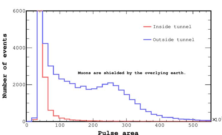
The muon peak identified (above). All muons are shielded by the overlying earth located underground at Hanbit NPP.
