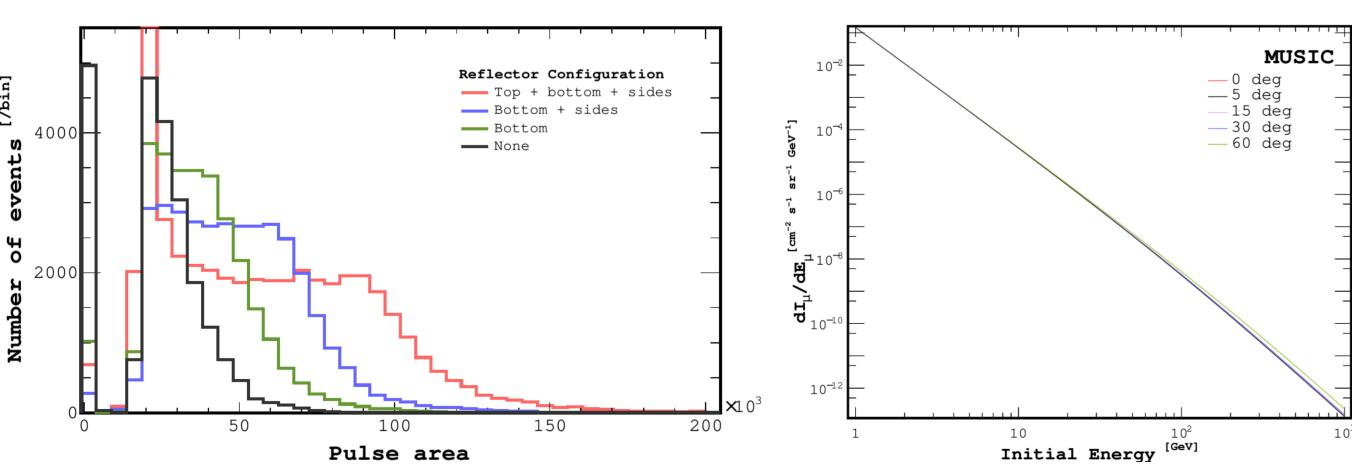
Detector light collection efficiency tests showed clear muon peaks (top left). MC simulation of muon flux reproduced muon event rates (top right).
