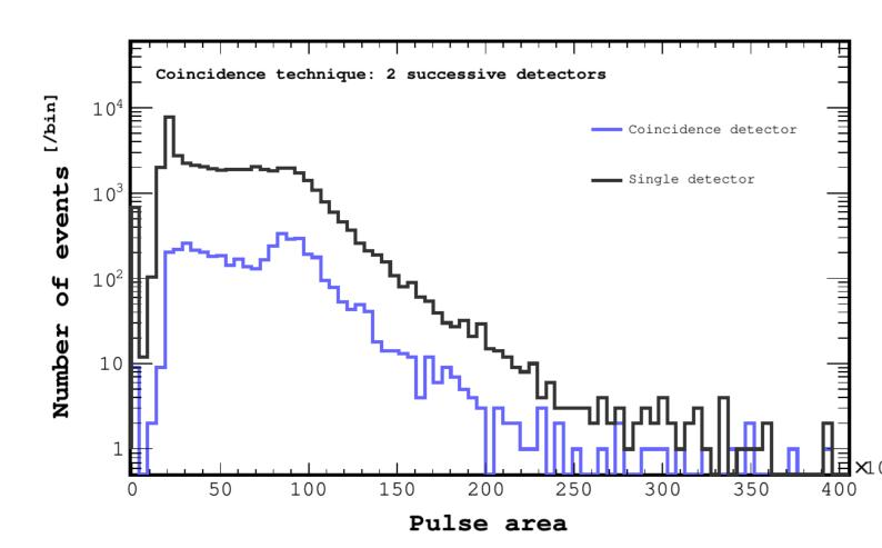
Using two stacked detectors in coincidence, we confirmed the peaks originate from cosmic muon scintillation events (bottom left).
