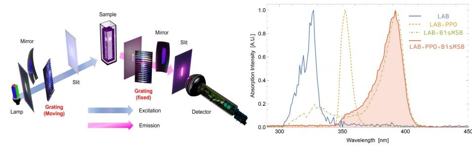
Explaining spectral differences between LAB+bis-MSB and LAB+PPO+bis-MSB samples via PPO-mediated FRET, considering the Stokes
