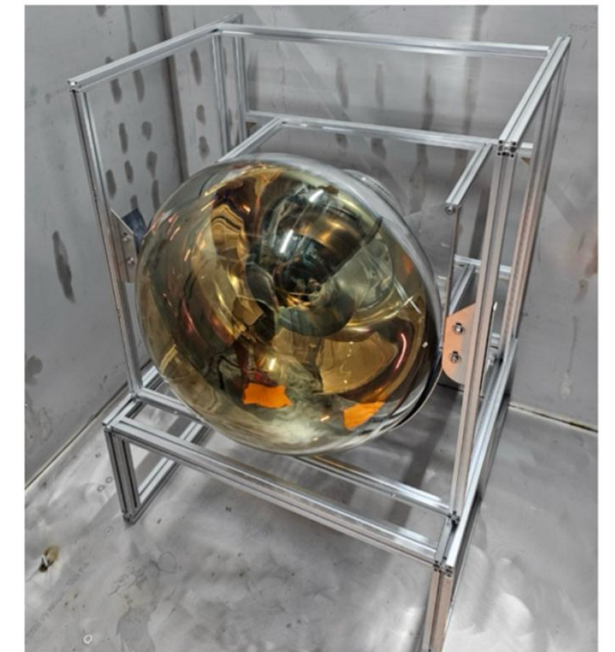
20-inch PMT (Hamamatsu R12860)
